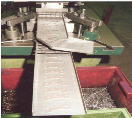
Above: Separation of scrap and finished parts through slots in the tray, letting the smallest details through into a box and the larger being transported into a separate box.
