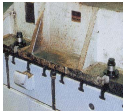
MC-Clamp for lower die, in clamped position
