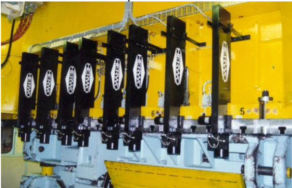
All HTC clamps in parking position.
