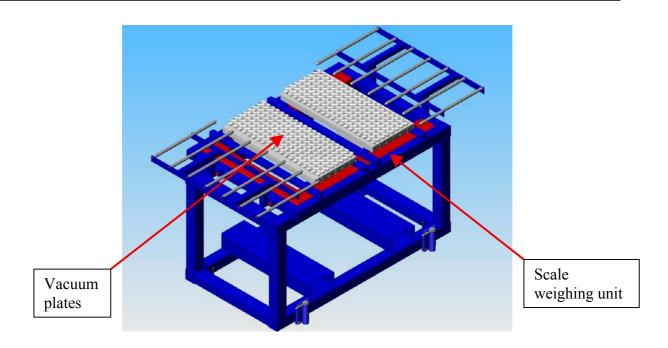
Data for weight of the panel is stored in the control system.
